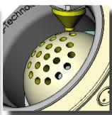
Specialized multi-axis Ruled features are used for operations that require continuous rotation. The match lines contained in the feature automatically control the synchronization of the wire throughout the cut.
